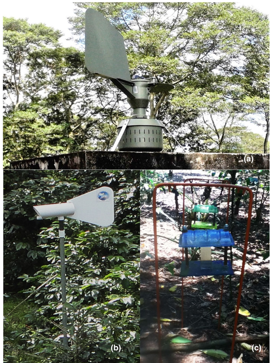
Fig. 1 a Hirst-type spore trap (HST). b Passive spore trap (PST). c Sediment spore trap (SSS).
